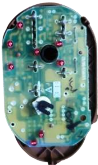
Figure 4. PCB soldering (vertical) position after improvement.
